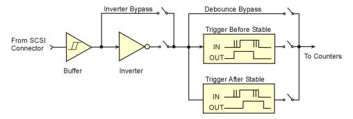
Figure 13. Debounce model block diagram
